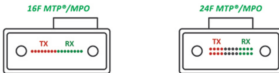
View into Transceiver, 400GBase-SR8 optical lane assignments
